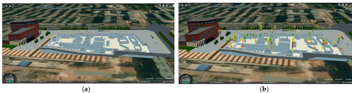
Figure 14. (a) Segmented model. The position of the internal hydrant parts can be clearly seen. (b) Fire hydrant parts coding. Three-dimensional grids of different colors represent the hydrant parts on different floors.
